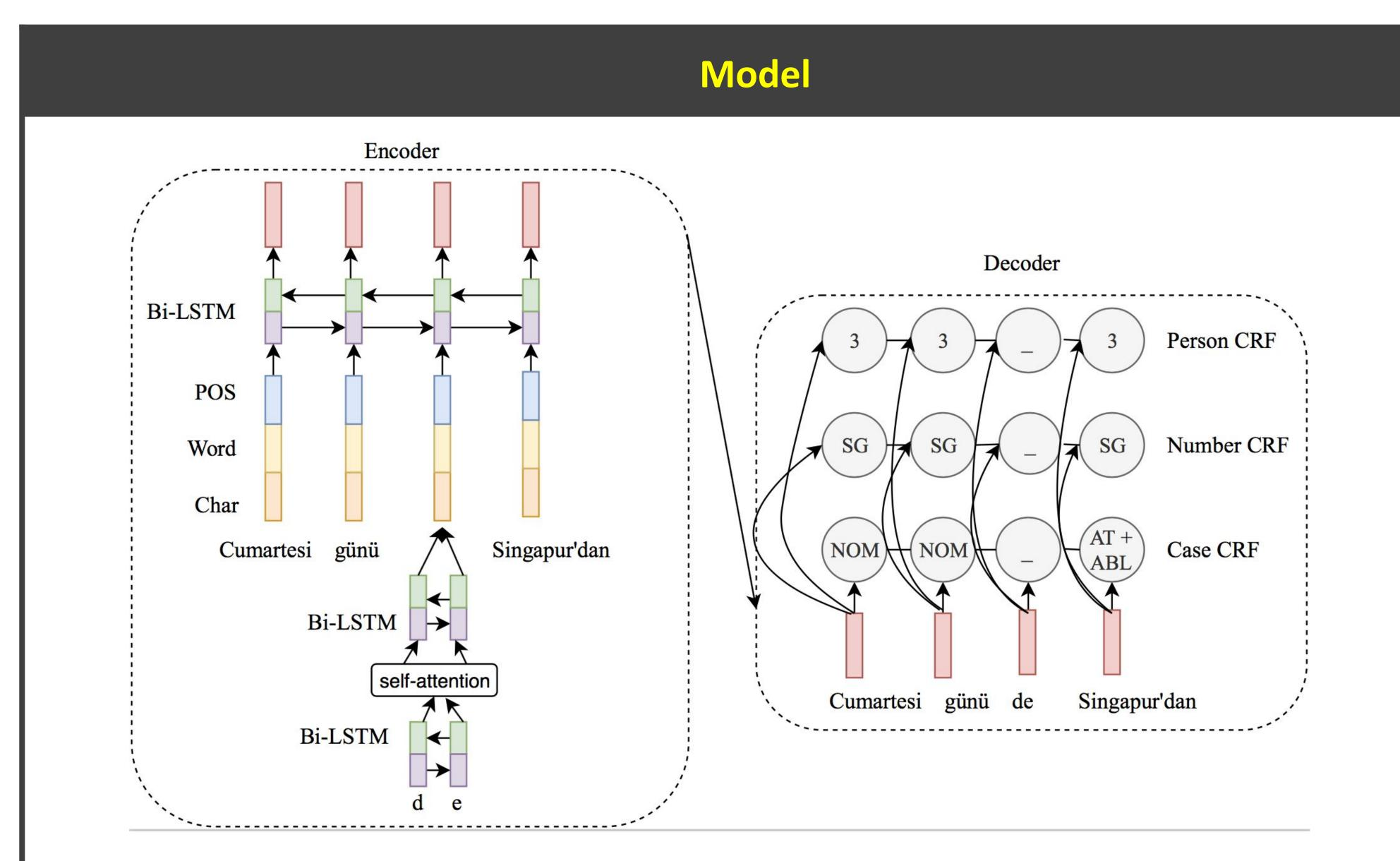
Hierarchical neural model for contextual morphological analysis with independent CRF decoders for each coarse-grained feature F such as Number, Person etc. POS embeddings are concatenated to the word and char-level representationse. This model has |F|-1 decoders since POS tagger is run separately as a prior step. MDCRF refers to the above model without POS embeddings having all |F| decoders.
